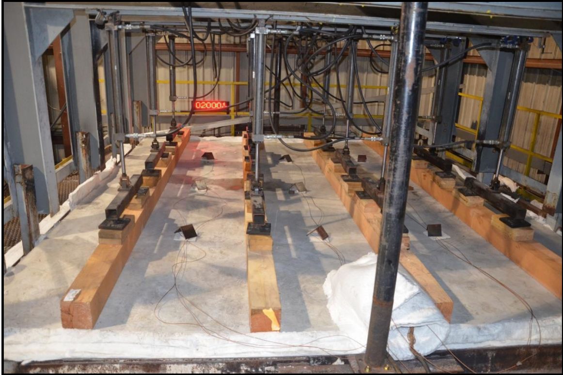
Figure B-7. Unexposed Face 2 h into the Test.
