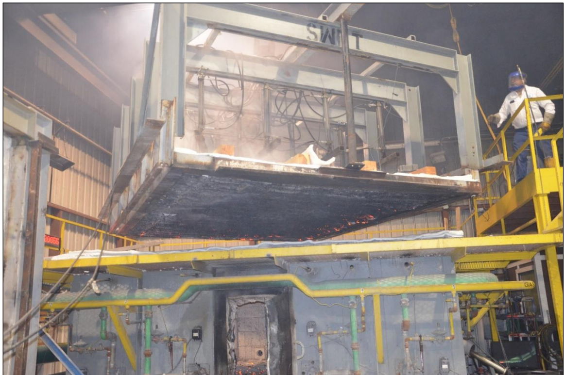
Figure B-8. Exposed Face upon Removal from Furnace.
