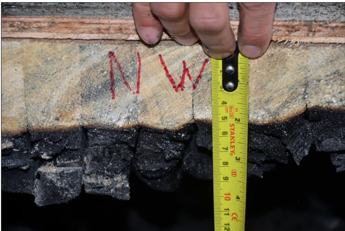
Figure B-10. Exposed Face Cross Section of the North West Quadrant after Chainsaw Cut.
